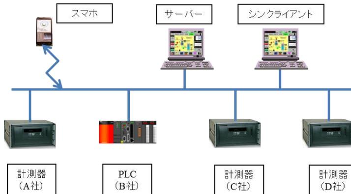
SCADA : supervisory control and data acquisition (監視制御とデータ収集)
